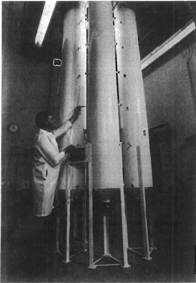
Fig. 2. Cages of test insects are inserted in metal silos (45 cm in diameter by 4.27 m high) containing 545 kg of wheat. Generated atmosphere is passed upward through the silos.
